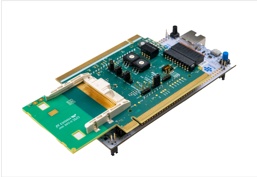
Figure 4. Assembly of adapter board and STM32 Nucleo-H753ZI
